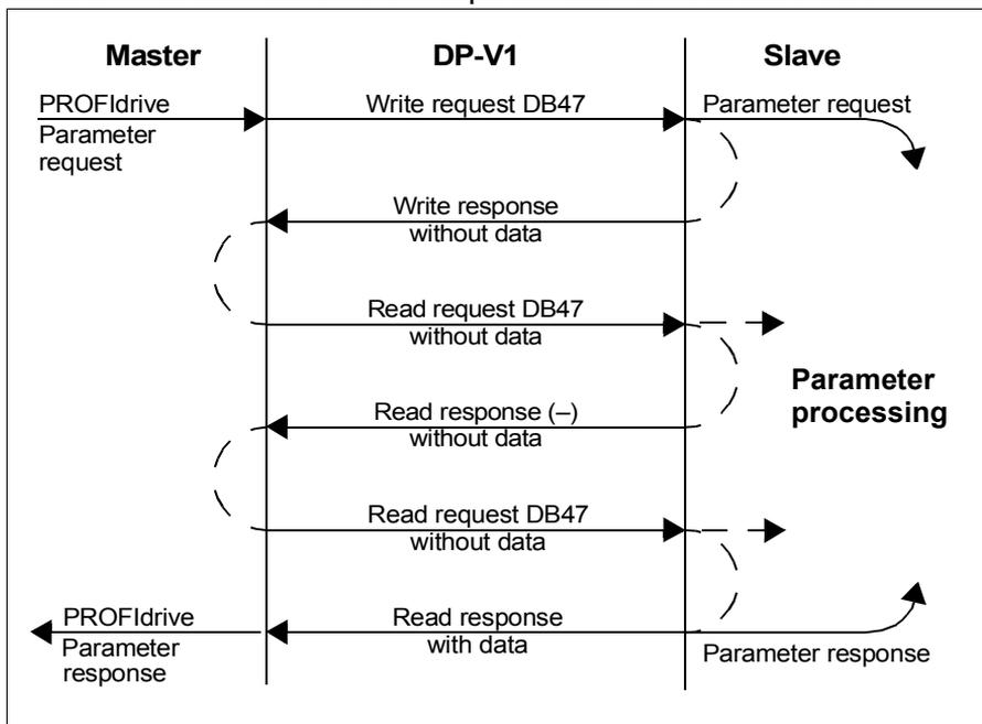
The messaging employs DP-V1 data units. The PROFIdrive parameter request is included within the DP-V1 request as data. Likewise, the DP-V1 response contains the PROFIdrive parameter response as data.
