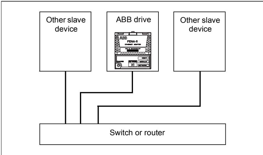
This figure shows an example of an allowable topology for an Ethernet network with FENA-21.
