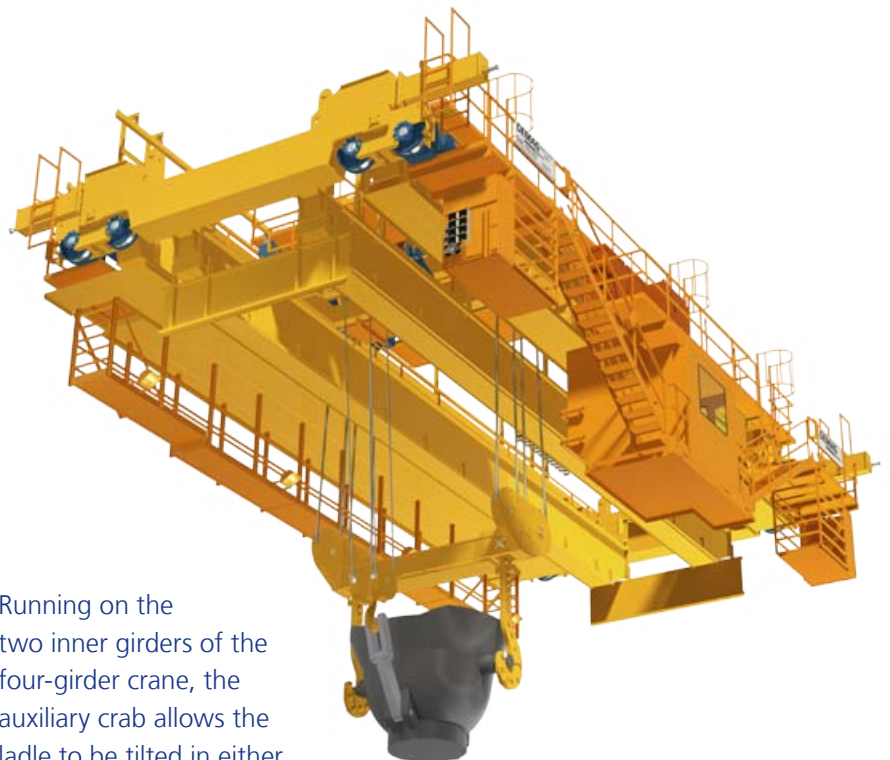
55/25-t four-girder overhead travelling crane for Mopani Copper, Zambia, span 18 m (photograph above, 3D illustration below and right)
