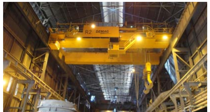
150/50-t two-girder overhead travelling crane for Arcelor Mittal, South Africa, span 24 m
