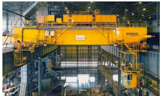
200/32/10-t two-girder overhead travelling crane for TISCOR, South Africa, span 22 m
