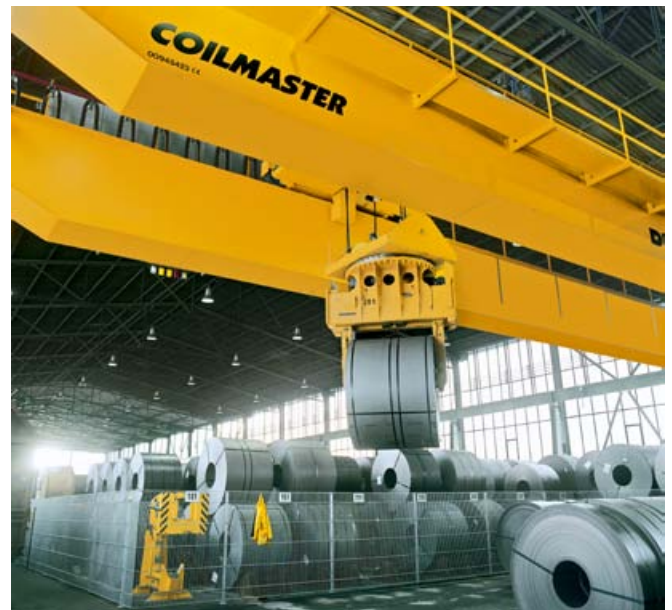
Coil handling in a cold-rolling mill in Germany: 36-t process crane with an automated storage area and inventory management system
