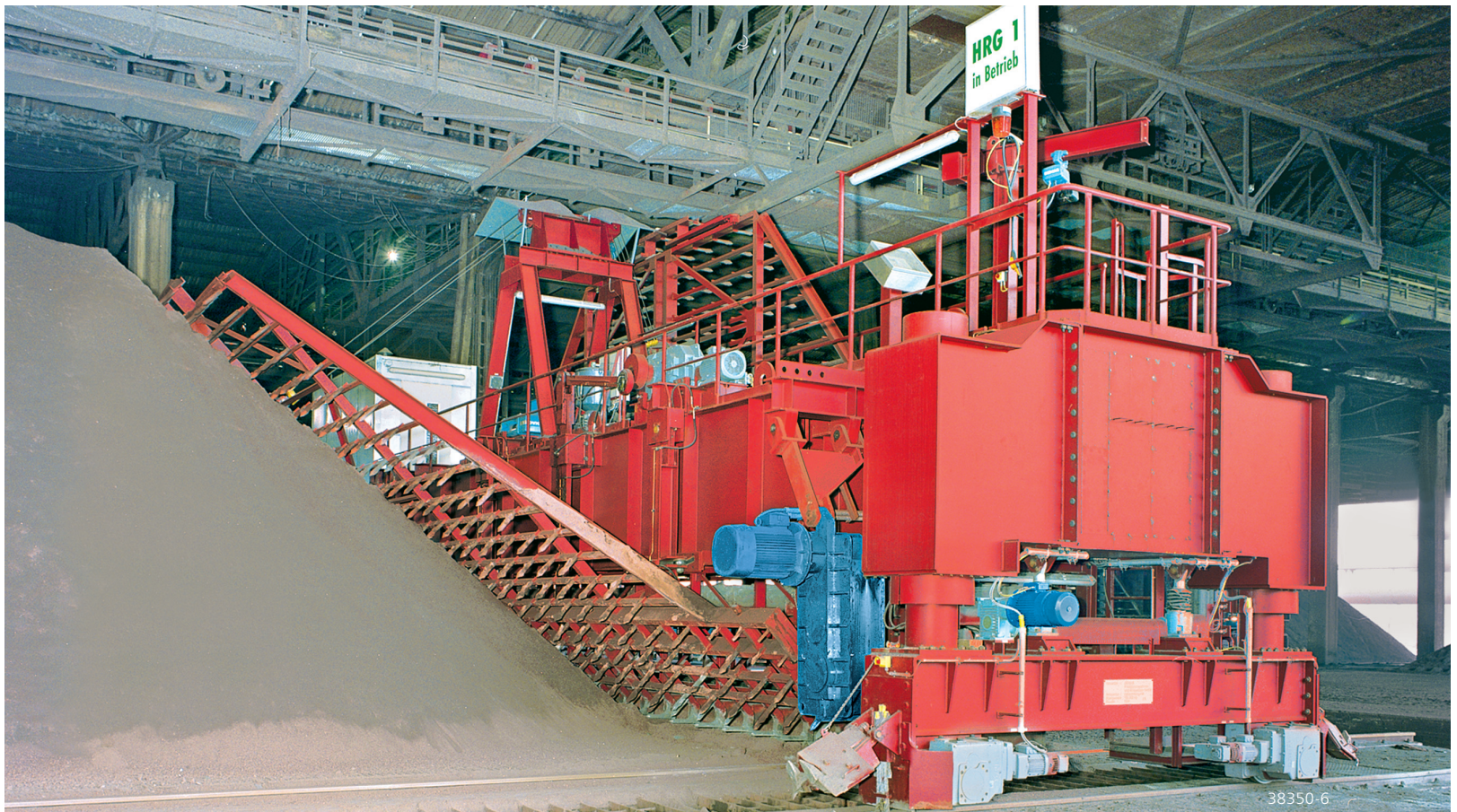
Angular geared motors drive a leveller
