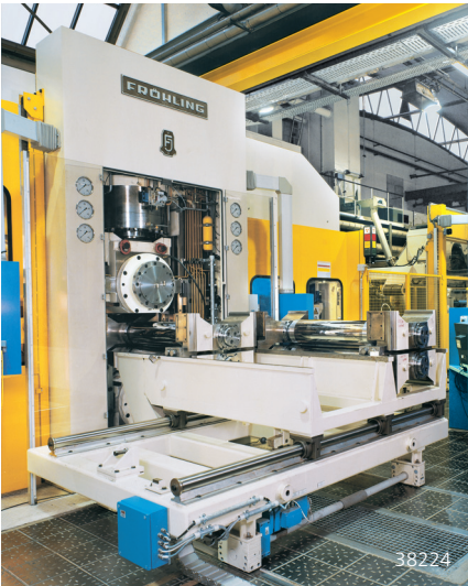
A tool-changing carriage is moved on wheel blocks driven by an offset geared motor operating as a central drive unit
