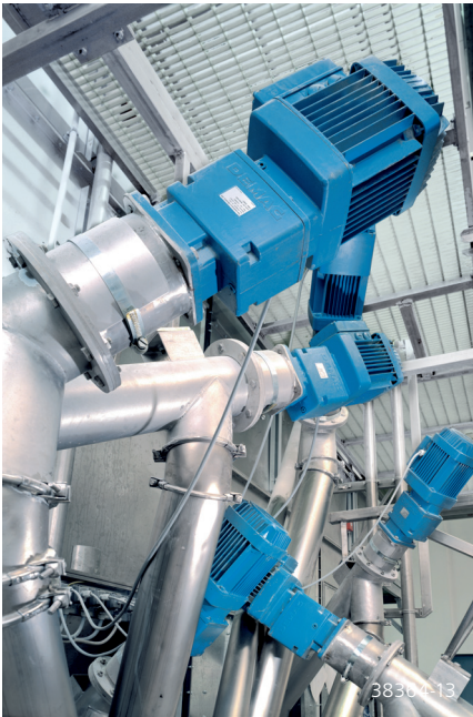
Helical geared motors drive the conveying screws of a feed system
