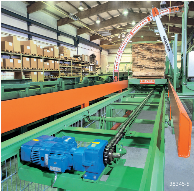
Microspeed drives are ideally suited as a robust drive for cutting lines in the timber industry
