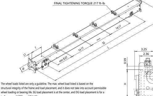
structural integrity of the frame and load placement, and it does not take into account permissible wheel loading or bearing life. SG load placement is at the center, and DG load placement is for a trolley gage of 1200 mm [47 1/4"].
