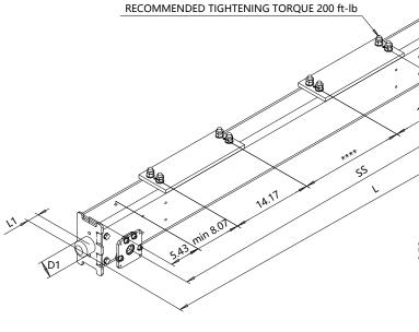
The wheel loads listed are only a guideline. The max. wheel load listed is based on the structural integrity of the frame and load placement, and it does not take into account permissible wheel loading or bearing life. SG load placement is at the center, and DG load placement is for a trolley gage of 1200 mm [47 1/4\*].
