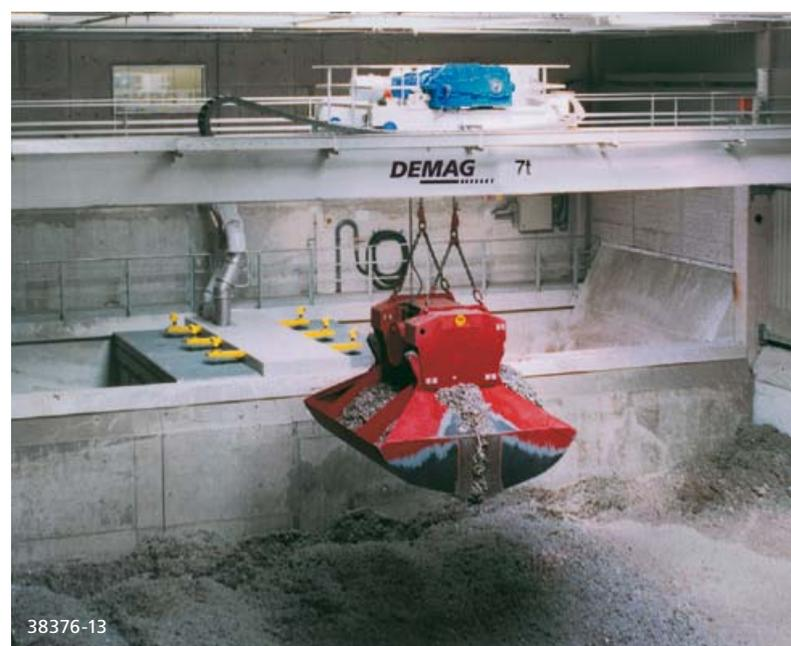
Demag automatic process cranes operating in a cement works
