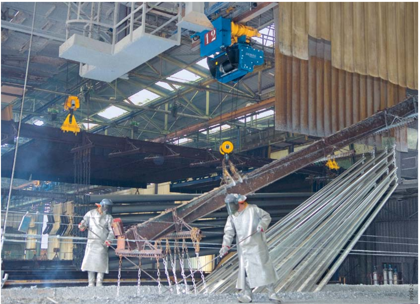
Demag FDR foot hoists travelling on a semi-automatic circuit in a galvanising plant.
