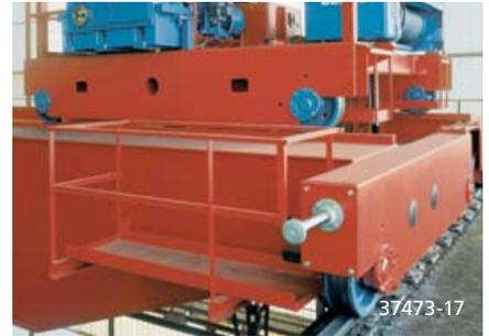
The wheel sets can be installed in hollow profile sections and box girder sections and as corner bearing units. Corner bearing arrangements offer the advantage of installing a pre-assembled wheel set in a travel unit without the need for extensive alignment. The unit can be rapidly replaced without the need for any alignment work, which ensures a high level of availability.
