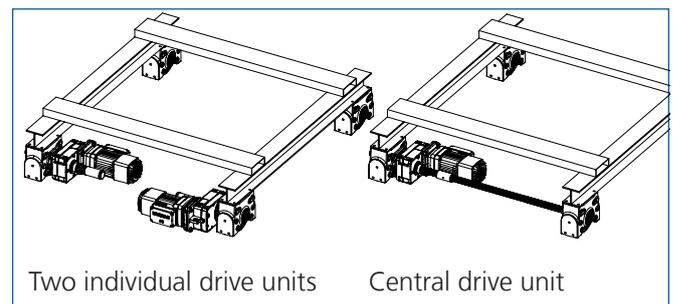
Various gearbox sizes are available with corresponding travel motors depending on the load to be moved and the required speed. Pole-changing geared motors can be selected from tables for line-fed operation (400 V, 50 Hz).
