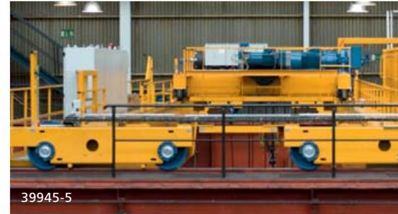
The use of these proven series-manufactured components offers a high level of functional reliability and guarantees interchangeability when the wheel is
