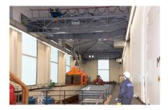
**41499-10:** Two double-girder overhead travelling cranes which each have a load capacity of 150 t and travel on a runway in the machine shop at the Albbruck-Dogern power station (RADAG) have been completely modernised by Demag Service.
