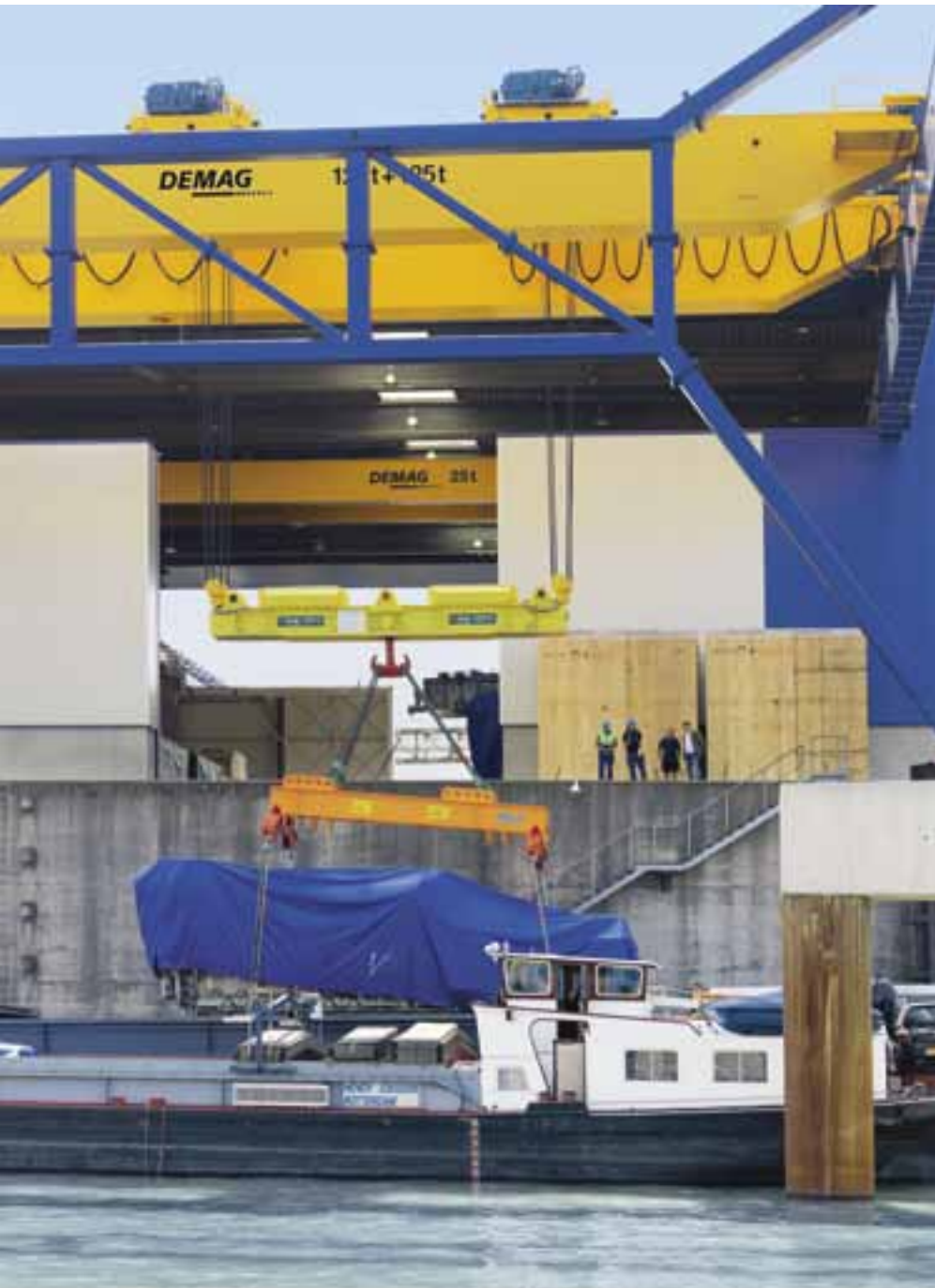
Cranes for the trimodal handling of heavy goods, e.g. generators
