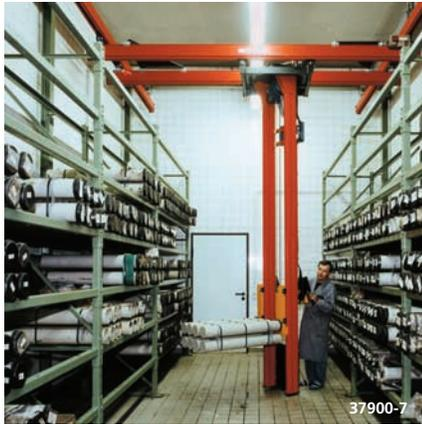
The lifting carriage can be fitted with forks, prongs, gripper tongs or other load handling attachments in accordance with the specific load handling requirements. The mast with its trolley is easily moved by hand and can rotate through 360°.
