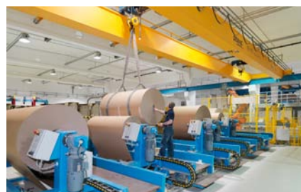
Overhead travelling crane above the packing machine
